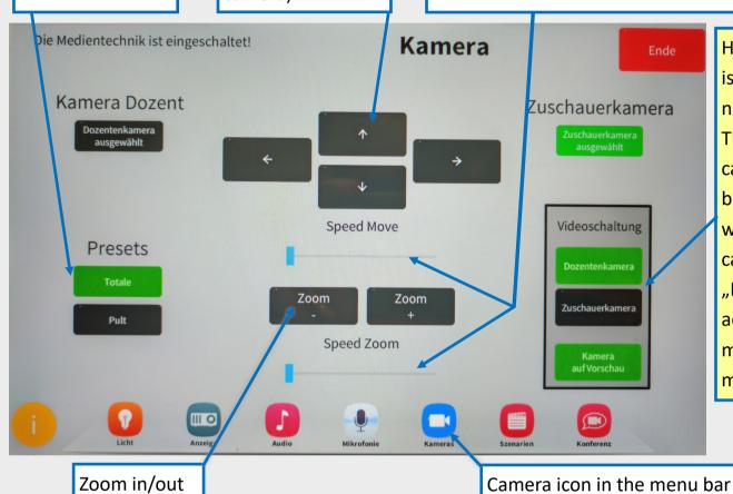
Here you define which camera is displayed on the preview monitor (monitor on the lectern). This signal is sent to the PC as a camera signal and can therefore be viewed as a webcam in the web conference. So that a camera image arrives at the PC, "Kamera auf Vorschau" must be activated and the camera image must be visible on the preview monitor.
